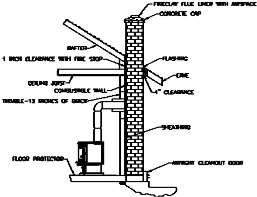
FIGURE 3.1 Connection to a Masonry Chimney (Exterior Shown)
