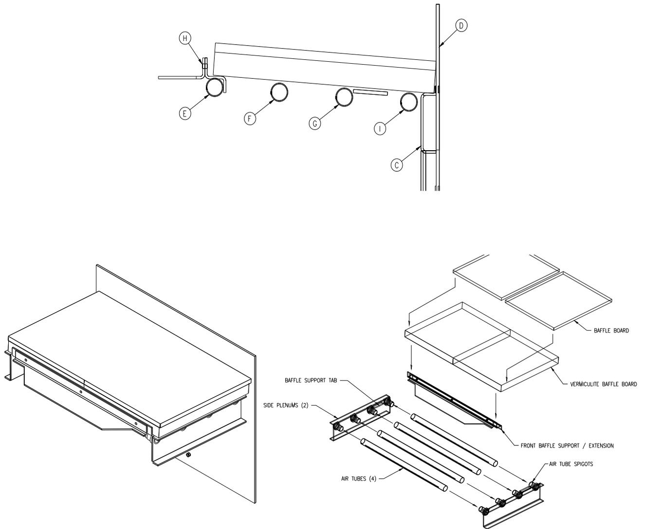
**FIGURE 9 – Baffle installation & removal**
