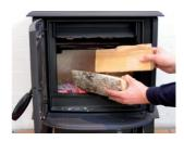
The stove door should normally be opened gently the first 2 - 3 centimetres, then you should wait until the pressure has equalised before opening the door all the way. This technique will prevent smoke from getting out, particularly when there is a poor draught.
