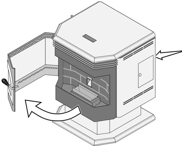
A keyhole is provided on the back of the stove to hang the door latch.
