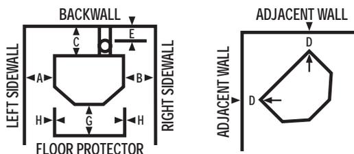
Maximum alcove depth 48 in/1220 mm, minimum ceiling height 60 in/1525 mm, minimum alcove width 44 in/1115 mm.
