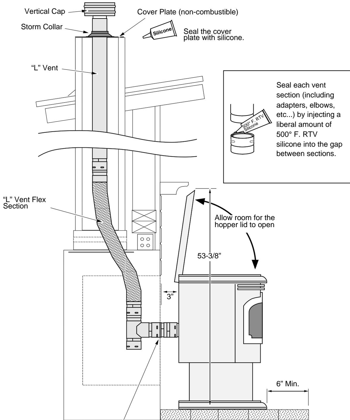
NOTE: you will probably need a short horizontal section here to clear the lintel and allow the hopper lid to open.
