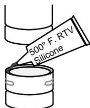
Seal each vent section (including adapters, elbows, etc...) by injecting a liberal amount of 500° F. RTV silicone into the gap between sections.
