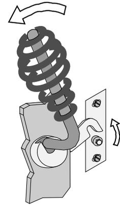
Turn the door latch counter-clockwise to disengage the latch.
