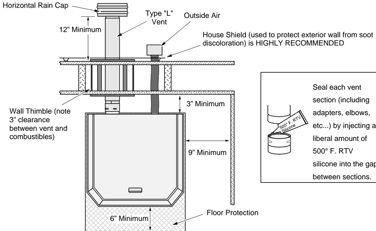
Seal each vent section (including adapters, elbows, etc...) by injecting a liberal amount of 500° F. RTV silicone into the gap between sections.
