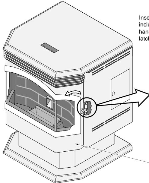
Insert the included door handle into the latch assembly.
