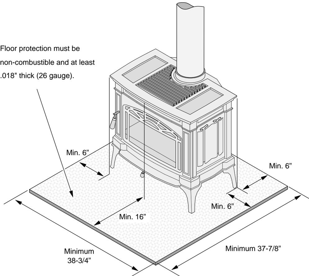
**NOTE:** In corner installations with reduced-clearance connector, the clearance to the wall is less than 6". In this case, floor protection must extend to the wall.
