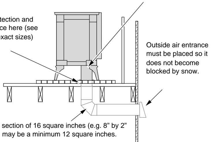
Maximum duct length is 15' with a cross section of 16 square inches (e.g. 8" by 2" duct). If under 5' long, the cross section may be a minimum 12 square inches.
