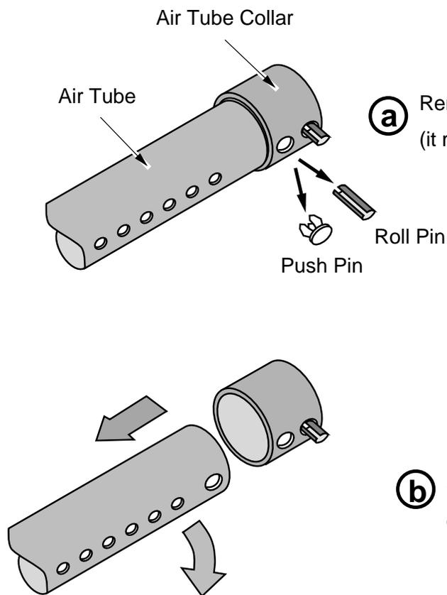
**a** Remove the left pin on the air tube collar (it may be a roll pin or push pin).
